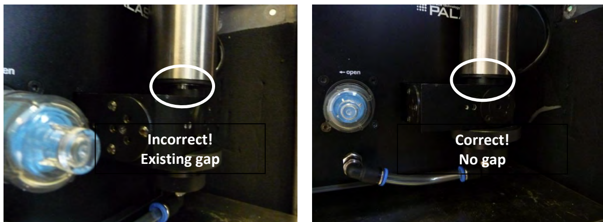
Fig. 18 A+B: on the left wrong position of the sampling tube, on the right correct position
