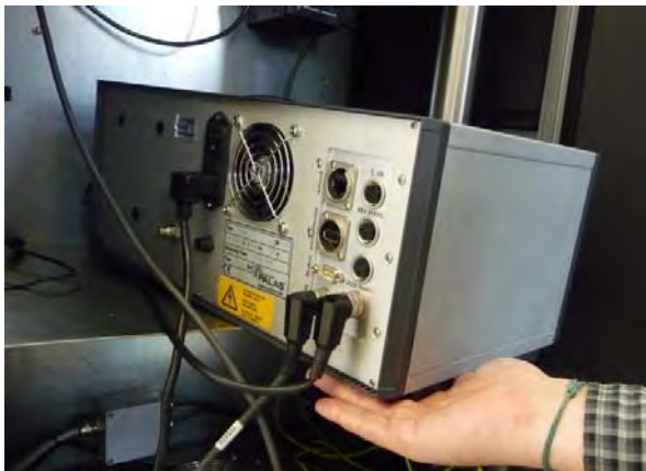
Fig. 16: Connection of the weather station, IADS with the ports on the back side
