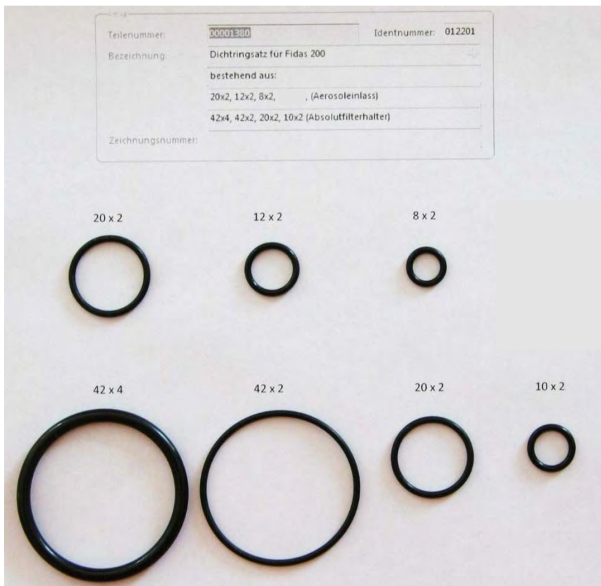
Figure 40: Sealing ring set for Fidas® 200
