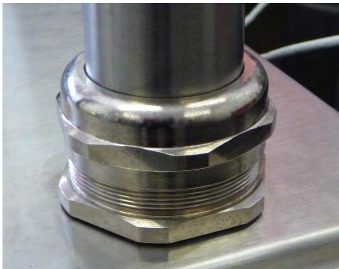
Fig. 9: Fixing of the weather station tube
