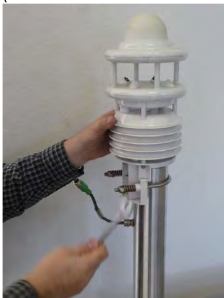
Fig. 10: Mounting of the weather station (here: WS600-UMB) at the tube
