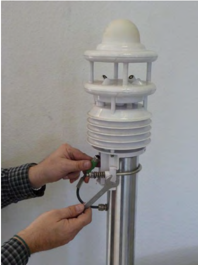
Fig. 11: Connection of the cable with the weather station
